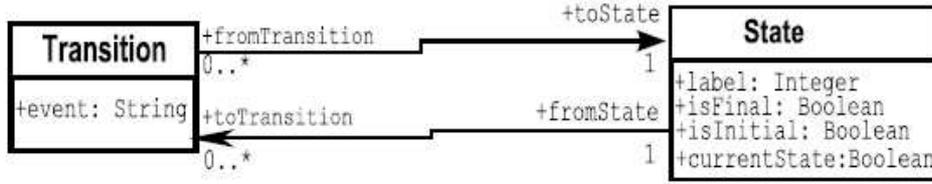
Fig. 3. The Finite State Machine Meta-model
