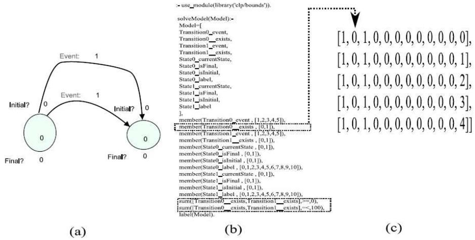
Fig. 5. (a) Association between **State** objects and a **Transition** (b) Generated CLP code (c) Cardinality constraint determines the value of an existence variable.
