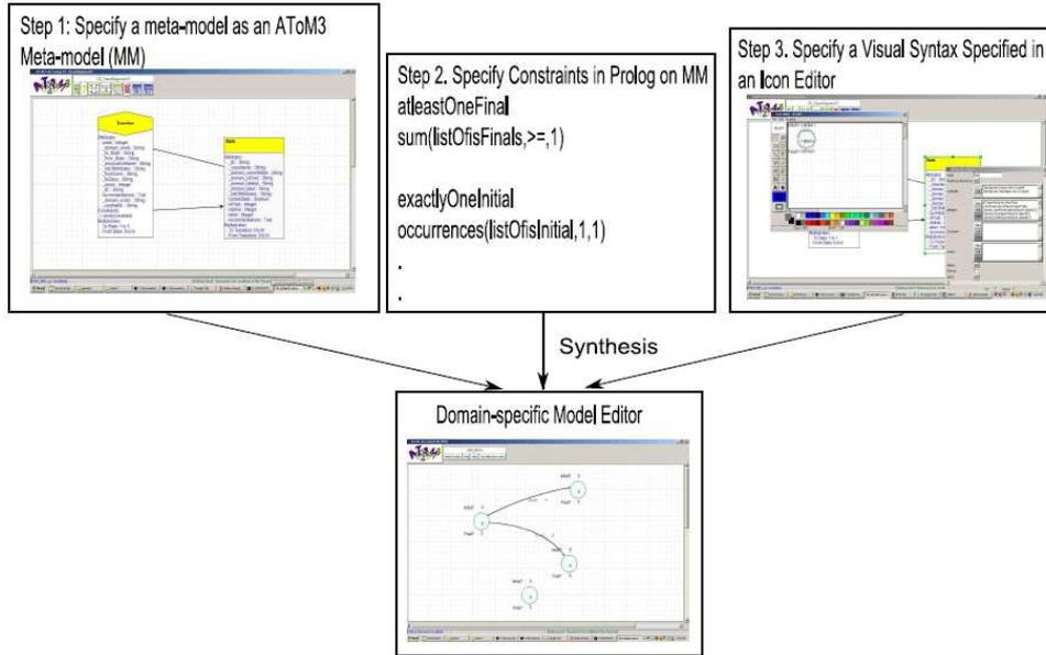
Fig. 1. Steps Taken by a DSML Designer to Synthesize a Model Editor in AToM<sup>3</sup>
