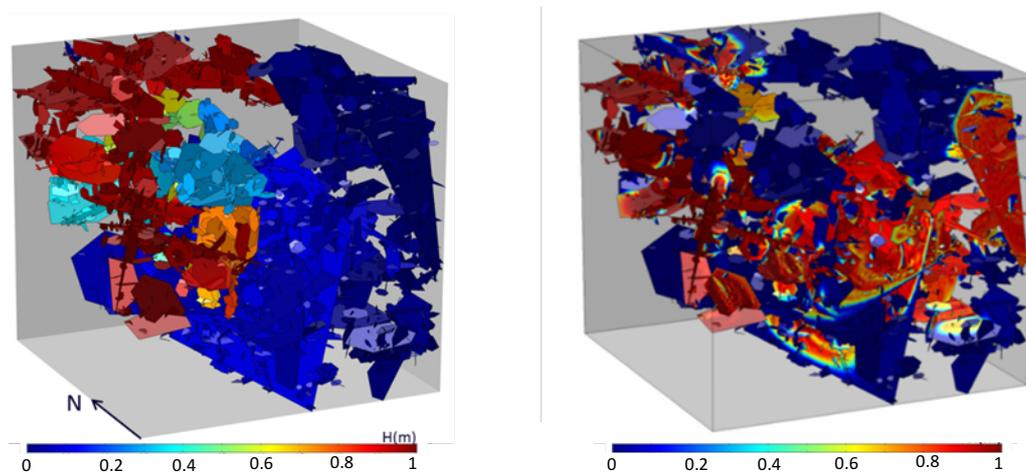
Figure 1: Hydraulic head (left) and tracer concentration (right) in a model with 3000 fractures.
