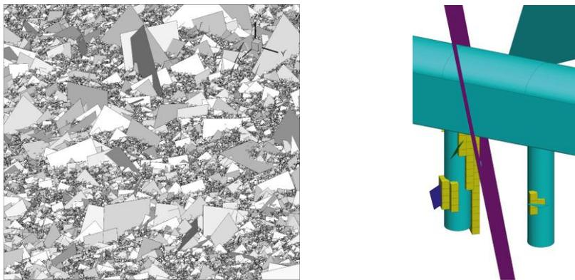
*Figure 3: Partial view of a 14M fracture network in repository analysis (left) and illustration of computational cells simultaneously in contact with deposition holes and fractures (right)*
