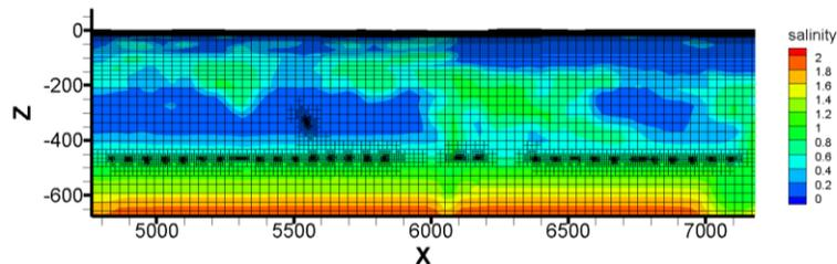
Figure 2: Example visualization of the computed salinity field before excavation of the Forsmark repository
