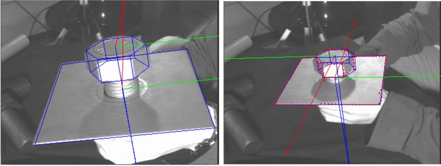
**Fig. 4.** Helical movement of a screw whilst the screw and the platform are simultaneously in movement. In this and all the following figures the reference frames for each component are shown as well as a projection of the CAD model onto the image. The axes of the frames are drawn in yellow, blue and red. The contour of the object is shown in blue. The points found to the normal of the contour are in red and the points rejected by the M-estimator are shown in green
