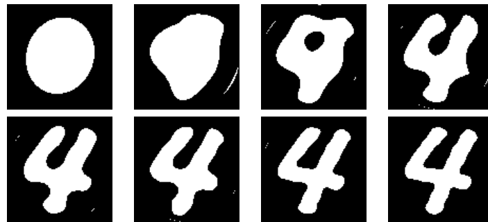
Figure 13: Progressive synthesis of the image of a digit 4, using its Zernike moments of order up to 2, 6, 8, 10, 12, 14, 18 and 20
