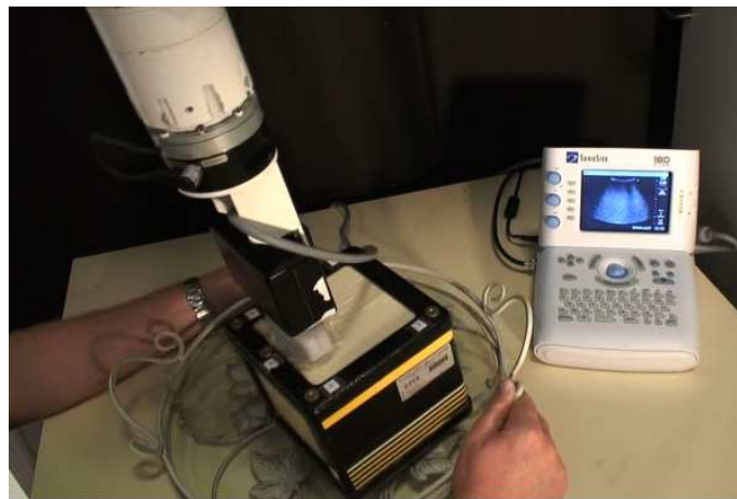
Figure 10. Automatic compensation of 6-DOF motions that are manually applied to an ultrasound phantom. The robotized ultrasound probe is controlled directly from the speckle contained in the observed ultrasound image.
