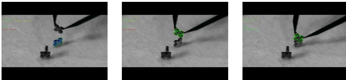
Figure 7. Micro assembly of two 400\mu\text{m} \times 400\mu\text{m} \times 100\mu\text{m} MEMS using visual servoing.
