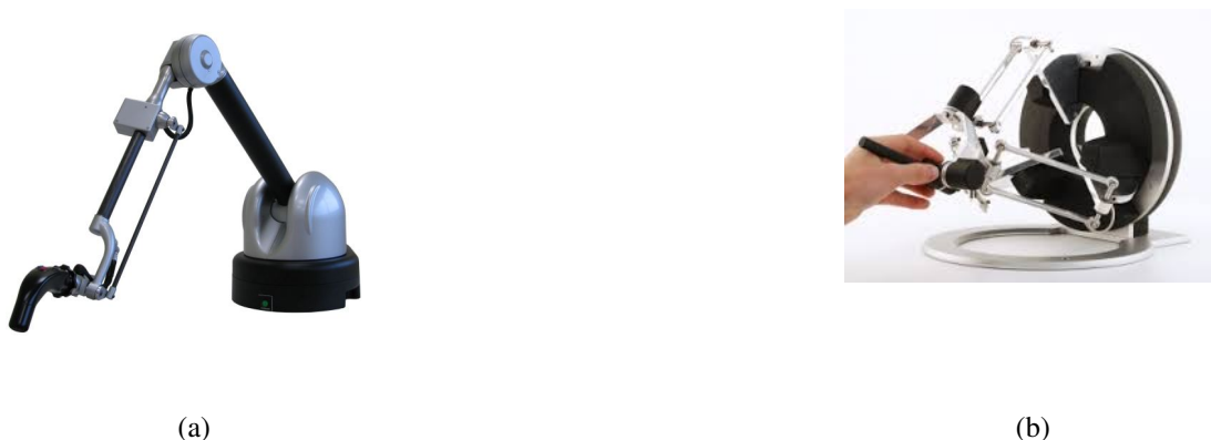
Figure 7. Haptics and Shared Control Platform. a) Virtuoso 6D and b) Omega 6 haptic devices
