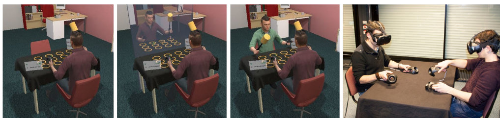
Figure 6. Setup of the experiment: each user was able to interact in the virtual environment with his own avatar, while the physical setup provided both a reference frame and passive haptic feedback. From left to right: experimental conditions Alone, Mirror and Shared; Physical setup of the experiment.
