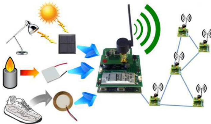
Figure 6: PowWow WSN Platform with Energy Harvesting
