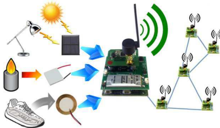
Figure 6: PowWow WSN Platform with Energy Harvesting
