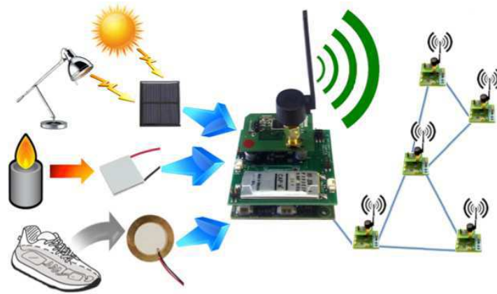
Figure 6: PowWow WSN Platform with Energy Harvesting
