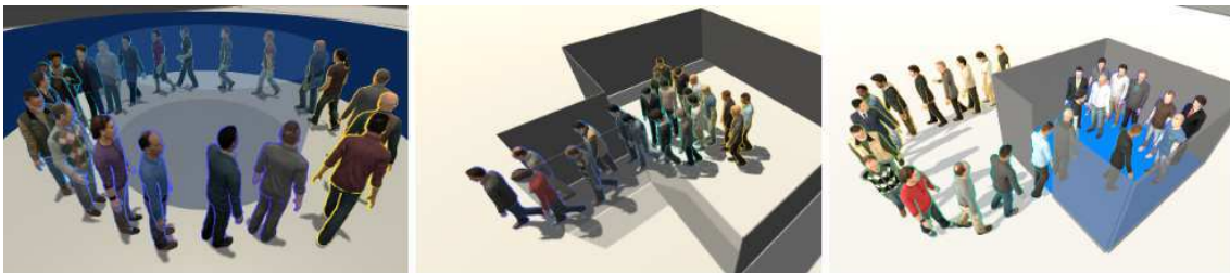
Figure 14: Snapshot of crowd motions generated using the one-man-crowd approach. A single user successively embodies each displayed virtual agent in the order indicated by the highlighting colour (from blue to yellow). We studied 3 scenarios that replicated existing experiments from left to right: circular unidirectional flow, bottleneck situation, inflow behaviour (entering a lift).
