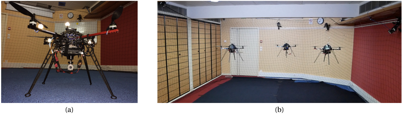
Figure 6: Unmanned Aerial Vehicles Platform. a) Quadrotor XL1 from Mikrokopter, b) Formation control with 3 XL1 from Mikrokopter in our flying arena equipped with the Vicon localization system.
