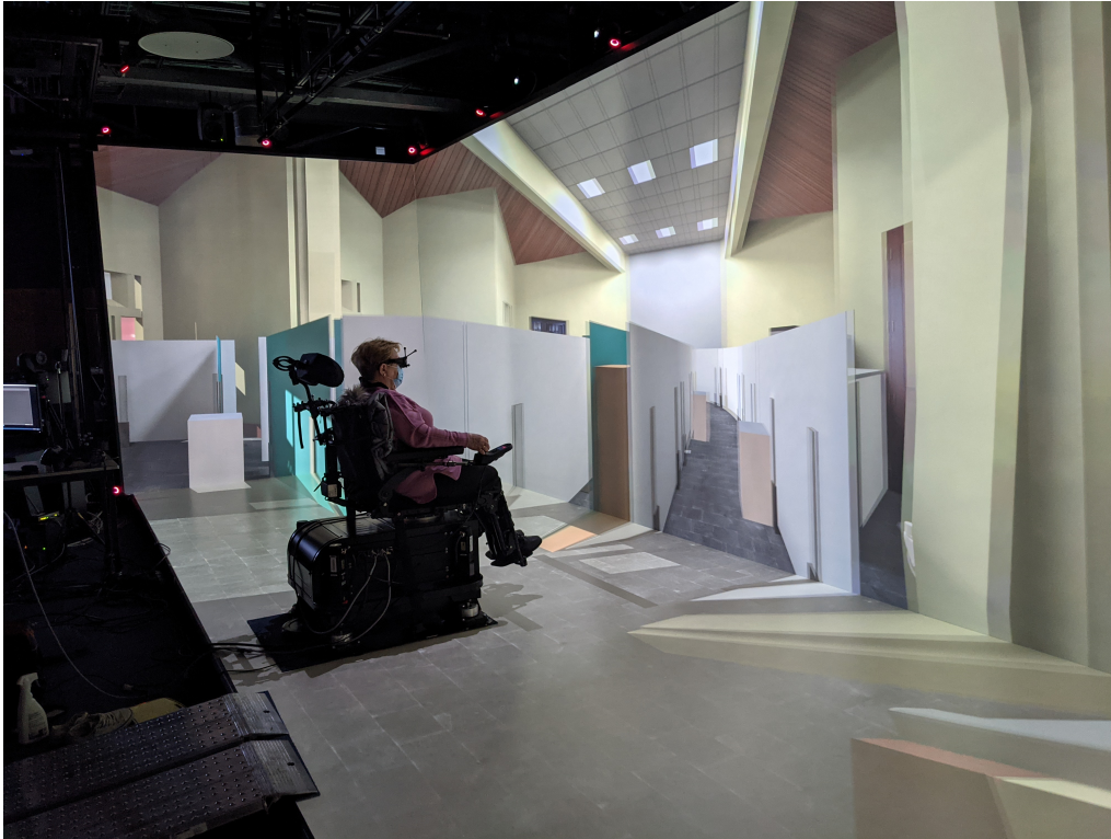
Figure 10: Participant driving in a virtual environment with our simulator and driving in real conditions with a real power wheelchair
