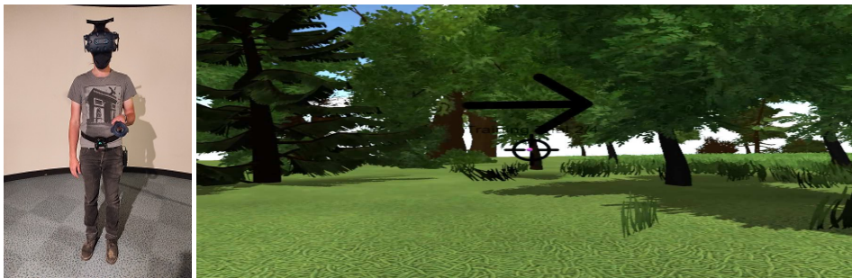
Figure 4: Left - User wearing the HTC Vive Pro Eye HMD equipped with a wireless module, one HTC Vive tracker located at the pelvis and one HTC Vive controller. Right - User's point of view of the VE during the experiment. The black arrow indicates the direction of the turn. The sight and pink sphere were used for calibration purposes).
