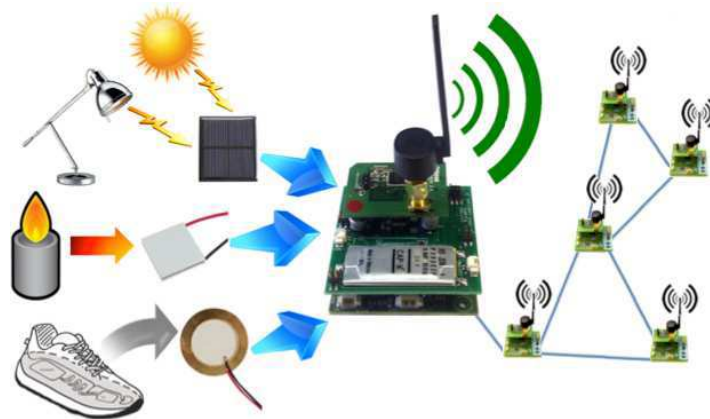
Figure 5: PowWow WSN Platform with Energy Harvesting
