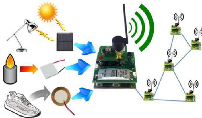
Figure 5: PowWow WSN Platform with Energy Harvesting
