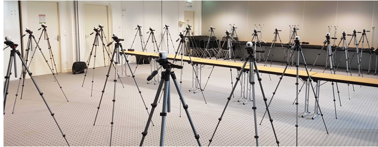
Figure 1. The 40 omnidirectional cameras positioned for an indoor scene capture.
