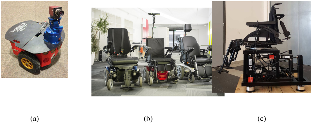
Figure 3. Mobile Robot Platform. a) Pioneer P3-DX robot, b) wheelchairs from Permobil, Sunrise and YouQ, c) the wheelchair haptic simulator.
