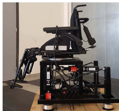
Figure 2. Upgrade of the Immersia platform: two new devices installed. (Left) "Scale-One" Haptic system for one or two users. (Right) Motion platform for powered wheelchair simulation.
