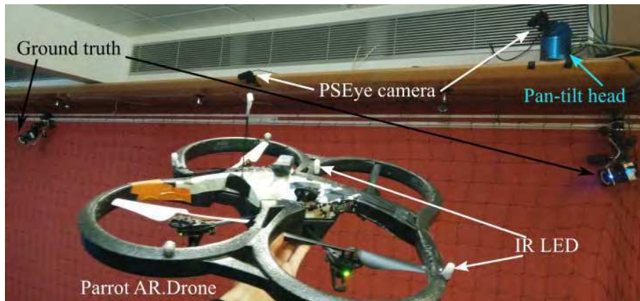
Figure 12. Our optical tracking prototype based on controlled cameras and hybrid stereo/single-view registration. The tracking is used for UAV indoor localization purposes.
