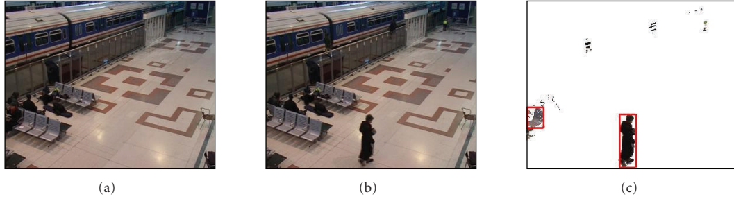
FIGURE 1: Observations obtained with background subtraction: (a) reference frame, (b) current frame, and (c) result of background subtraction (pixels in black are labeled as foreground) and derived object detections (indicated with red bounding boxes).
