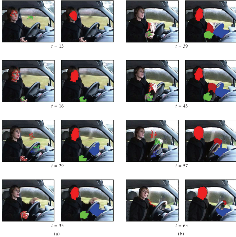
FIGURE 11: Results on a driver sequence. The observations are moving clusters detected with the method in [2]. At each time instant, the observations are shown in the left image, while the masks of the tracked objects are shown in the right image.
