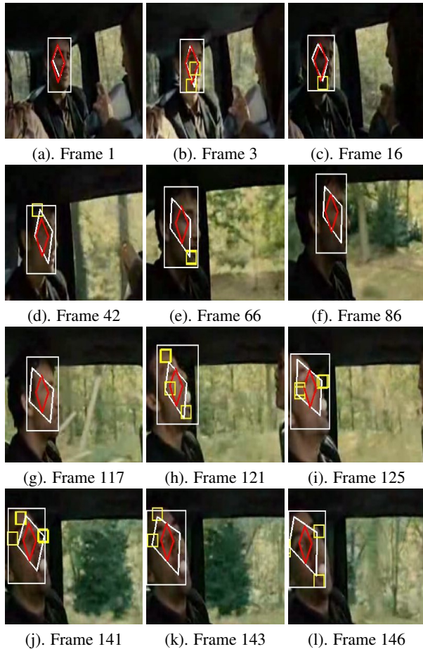
Figure 8. Results on the Children of Men sequence. This video has poor recording quality. Large motion jerks eventually cause tracking failure.
