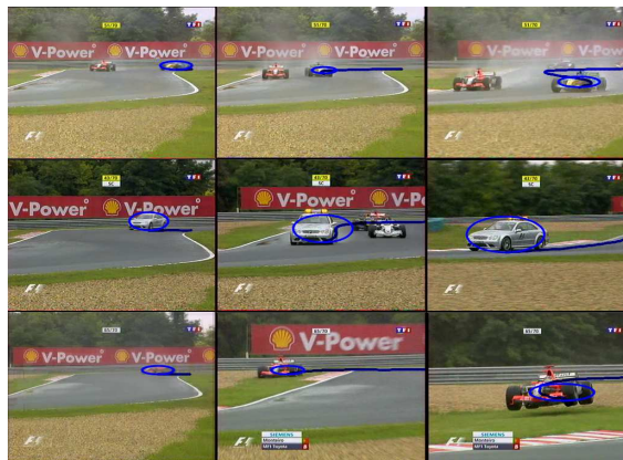
Figure 5: Images from Formula One race video shots acquired by the same camera. Top row: images displaying instances of a regular class. Bottom rows: example of unexpected events (safety car, car driving off the track). The trajectories are overprinted on the images.
