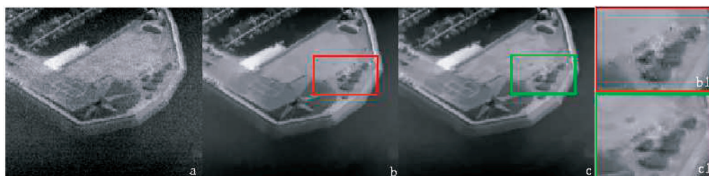
Fig. 7. Infrared sequence. (a) One image of the original sequence. (b) The corresponding image of the denoised sequence with the nonlocal means filter applied with a patch of fixed size 5 \times 5 pixels and the bandwidth equal to four times the noise standard deviation. (c) Denoised image with the proposed motion compensated filter, (b1) Cropped region of (b) and (c1) Cropped region of (c).
