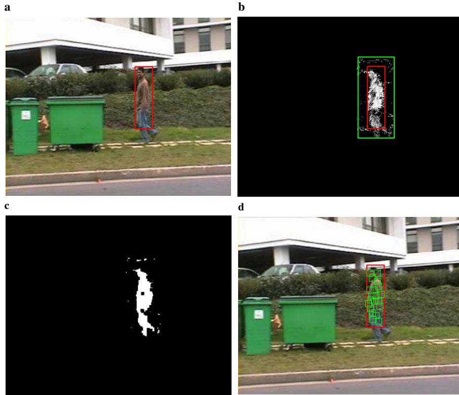
Fig. 4. Track point initialization using T_0 : (a) Initial frame with object boundary (b) likelihood map T_0 (c) Mask obtained after morphological operations (d) tracking points with the support region. Here, the number of tracking points is 20 with a support region of 100 pixels.
