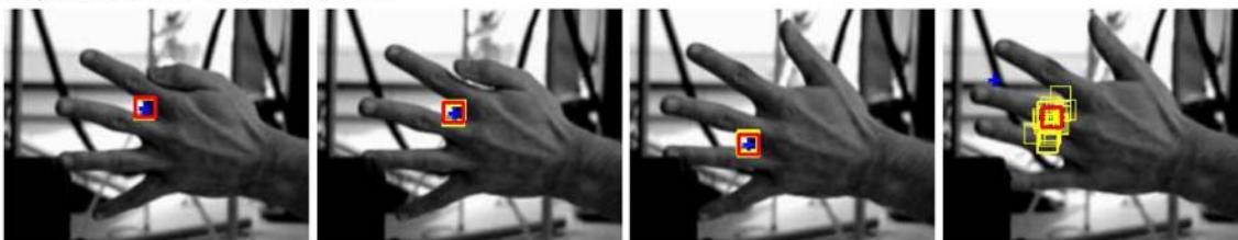
(b) Tracking result of the point situated between the forefinger and the middle finger. Use of the simple tracker, considering only one measurement. This observation is represented in blue, the feature location estimate in red and the set of particles in yellow (100 particles have been used) – frames 2, 7, 15, 19
