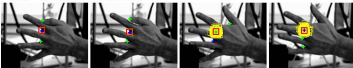
(d) Tracking result of the point located between the forefinger and the middle finger. Use of the tracker dedicated to ambiguities, considering three measurements. The first observation (corresponding to the highest correlation score) is represented in blue, the two secondary measurements are in green. The feature location estimate in red and the set of particles in yellow (100 particles have been used) – frames 2, 7, 15, 19
