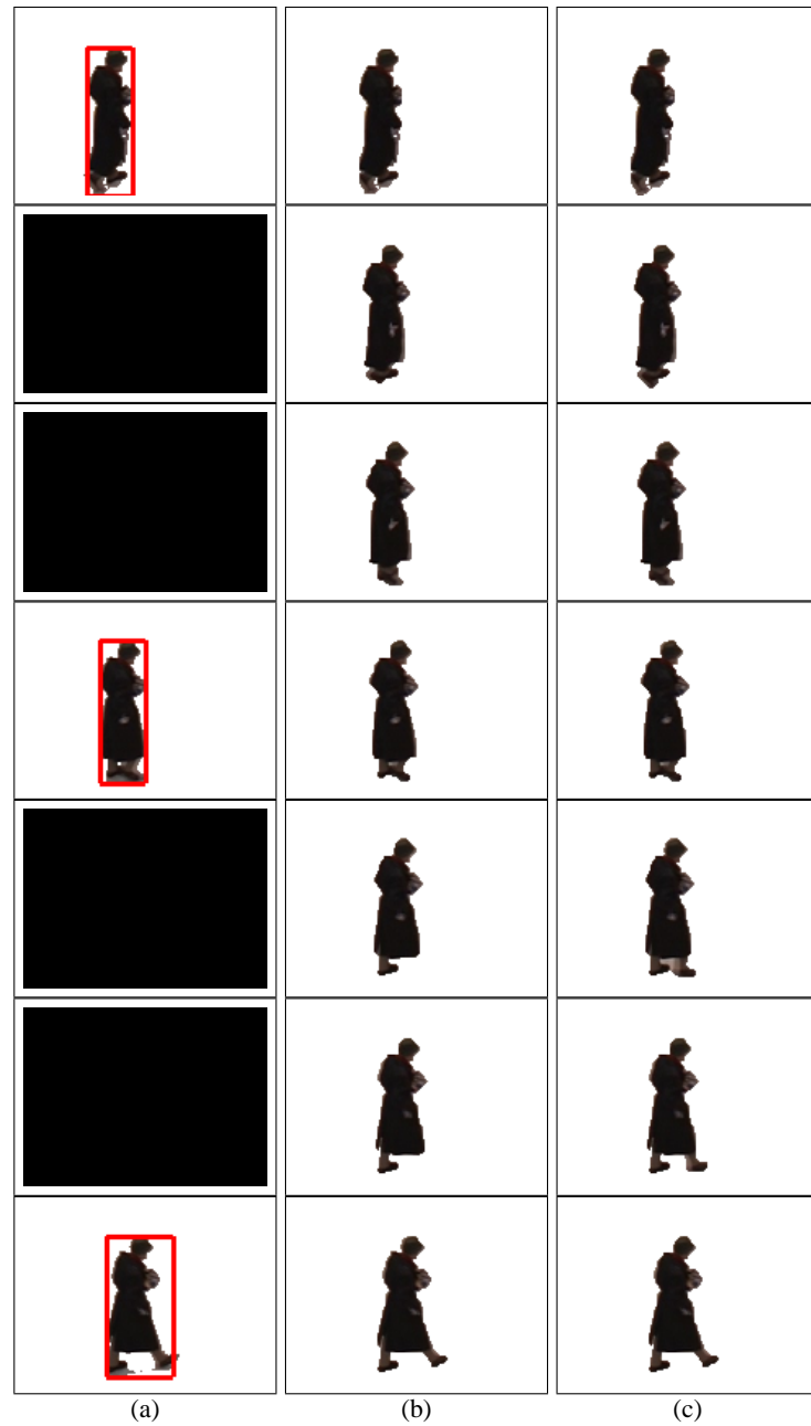
Fig. 8. Results with observations only every 3 frames on the PETS 2006 sequence for frames 801 to 807 (a) Result of background subtraction and observations (b) Masks of tracked and segmented objects (c) Comparison with the masks obtained when there is no missing observations
