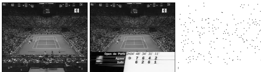
Fig. 4. Robustness to occlusion. Despite the partial occlusion the two images are detected as very similar with confidence value of -\log_{10}(NFA) = 50.1 . The right plot gives the position of the 200 sample points. There are not points in constant areas (because of the gradient threshold). However, some points are selected in the non-matching area (scores), but the NFA is still very low.
