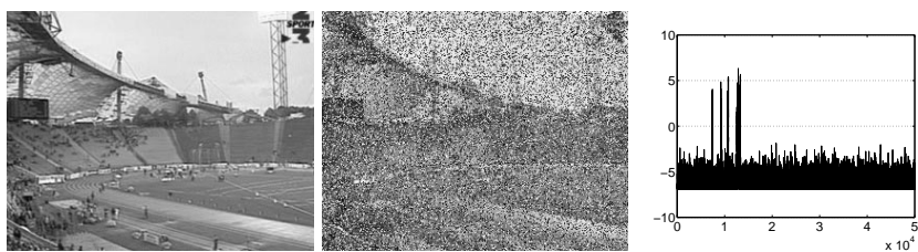
Fig. 2. The middle image is a 50% impulse noise version of the original one. In a database of 10^5 images, they still match with a NFA close to 10^{-5} . The right plot shows the confidence values (-\log_{10}(NFA)) for the first 50000 images of the sequence, the query being the noisy image. The peaks indeed correspond to exactly the same view of the stadium.
