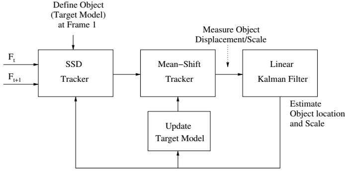
Fig. 1. Overview of the proposed tracking system
