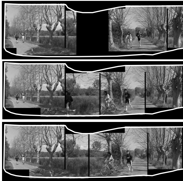
Fig. 5. Comparison of the selection of the key-frames obtained with the three methods applied to the S5 sequence. White line delimits the geometric manifold we want to cover. Top row: temporal sampling method; middle row: direct method, bottom row: iterative method. The images of the selected key-frames are displayed. N^*=4 .
