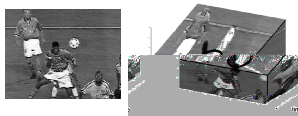
Figure 1: Result of detecting the strongest spatio-temporal interest point in a football sequence with a player heading the ball. The detected event corresponds to the high spatio-temporal variation of the image data or a “space-time corner” as illustrated by the spatio-temporal slice on the right.
