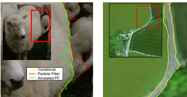
Figure 6. Contour extraction. Comparison of the different tracking algorithms on a difficult single contour extraction problem (left), and variational twofold contour extraction in an aerial photograph (right).
