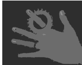
e. Piecewise-constant approximation using \lambda = 0.025 \times 255^2 ( P = 7 ) (entropic quantization)
