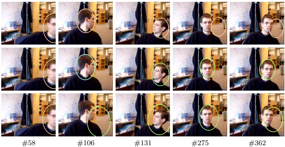
Fig. 3. Tracking results with adaptation disabled (top), enabled (middle and bottom) and the frame-difference likelihood disabled (bottom). The object is successfully detected (#58) and tracked during periods of motion (#106, #131) if the frame-difference likelihood is enabled (top, middle). With the object stationary (#275, #362) track is lost in the non-adaptive case (top) due to the skin-coloured carpet in the background, whereas the individualised model maintains lock (middle). With the frame-difference likelihood disabled (bottom) lock is soon lost and the colour model drifts to the background.
