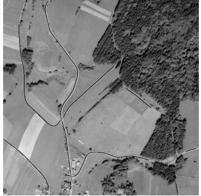
Fig. 13. Road extraction in image “Marchetsreut” (centerlines only)
