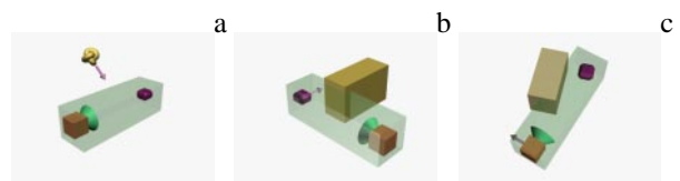
Figure 1: Occlusion issues (a) occlusion due to a moving object (b) occlusion due to the target motion (c) occlusion due to the camera motion
