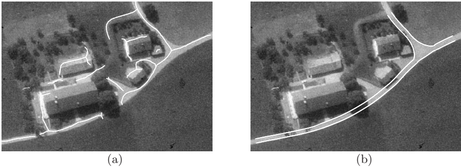
Fig. 8. Road extraction for a complicated scene (a) Line extraction (b) Final result
