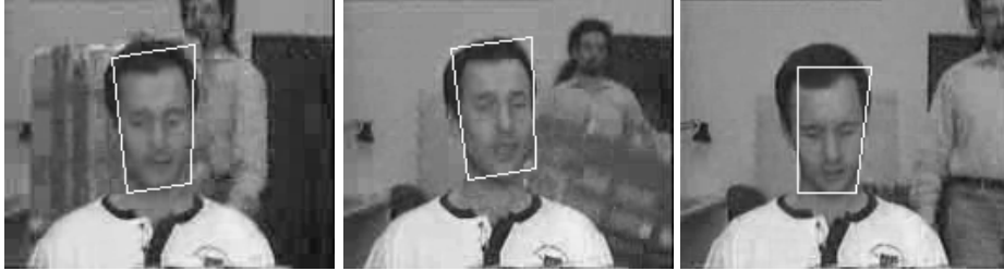
Fig. 2. GLR face detection on 4 intermediate frames of a QCIF videophone sequence (perspective transform).
