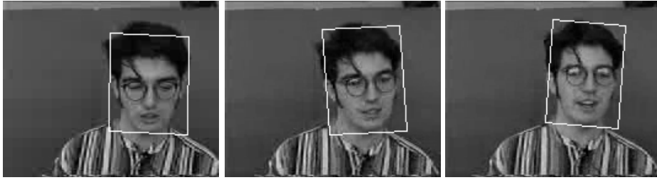
Fig. 1. GLR face detection on 4 intermediate frames of a QCIF videophone sequence (affine transform).
