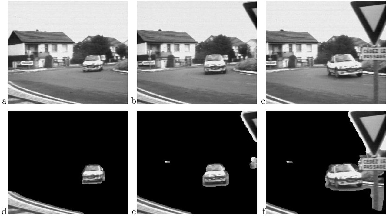
Figure 4: a) b) c) Roundabout sequence images at time: a)  $t_{58}$ , b)  $t_{62}$ , and c)  $t_{66}$ . d) e) f) Detection maps obtained at time: d)  $t_{58}$ , e)  $t_{62}$ , and f)  $t_{66}$ .
