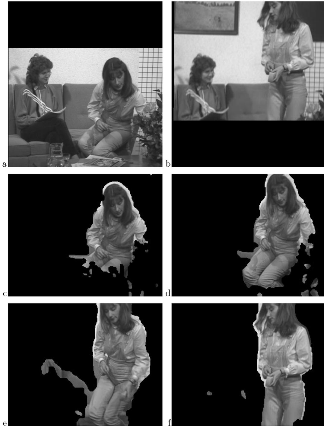
Figure 3: Sequence “interview” a) image at time  $t_1$ ; b) image at time  $t_{43}$ , compensated by the estimated dominant motions. c-d-e-f) Detection maps obtained at time: c)  $t_1$ , d)  $t_{13}$ , e)  $t_{25}$  and f)  $t_{43}$ .
