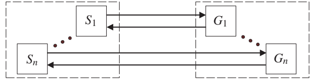
Fig. 4. Structural decentralized architecture
