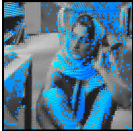
Figure 2: Image predicted with MP (left), image predicted with GMF (right). Blocks in blue are those selected with the SSE criterion, compared to the 9 modes of H264.
