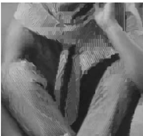
Figure 3: Image predicted with the 9 directional modes of H264/AVC (left), image predicted with AVC modes and GMF (right)
