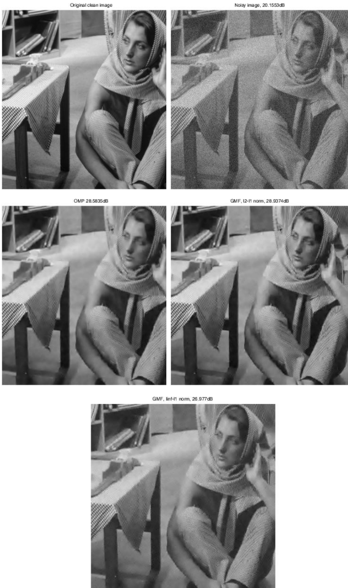
Fig. 1. Denoising with three sparse representation techniques: OMP (Orthogonal Matching Pursuit), GMF (Global Matched Filter) with the \ell_2 - \ell_1 criterion, and GMF with the \ell_\infty - \ell_1 criterion, for an AWGN ( \sigma = 25 ).
