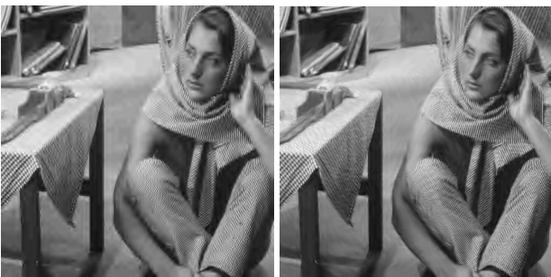
Fig. 5. [left] 3-level separable 9/7 wavelet coding of barbara 512x512 at 0.3 bpp, PSNR = 26.93 dB. [right] 6-level oriented 9/7 wavelet coding at 0.3 bits/pixels, PSNR = 28.24 dB. The low pass band has the same resolution in both cases.
