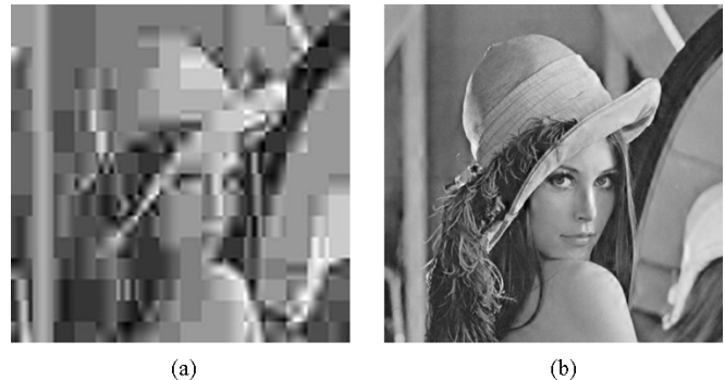
Fig. 10. Comparison between the two pirated Lena images. This is their best quality for a successful attack. Pirate A: PSNR = 21.8 dB, Pirate B: PSNR = 35.8 dB. (a) Pirate A. (b) Pirate B.
