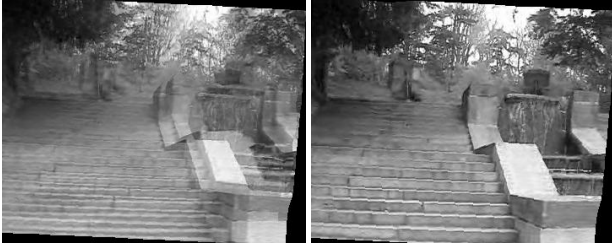
Fig. 7. Effect of geometric morphing on Stairway sequence: to visualise the geometric shift, two successive models are projected and superimposed for a viewpoint outside the camera path, without geometric morphing (left) and with geometric morphing(right).
