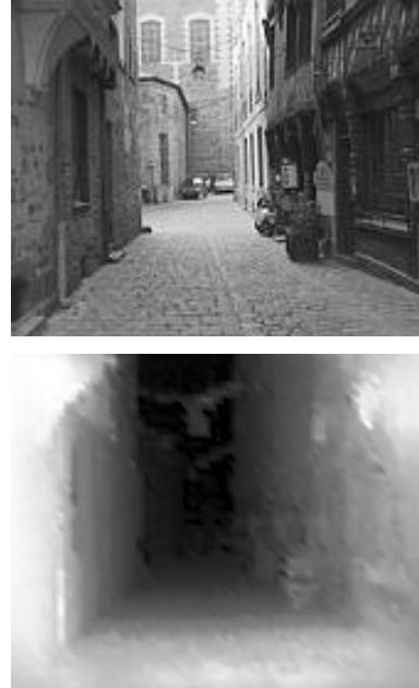
Fig. 2. An example of a depth map (bottom) extracted from the Street video sequence. The top figure is the corresponding image in the sequence.
