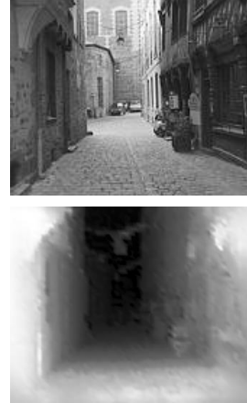
Fig. 2. An example of a depth map (bottom) extracted from the Street video sequence. Pictures on top is the corresponding image in the sequence.
