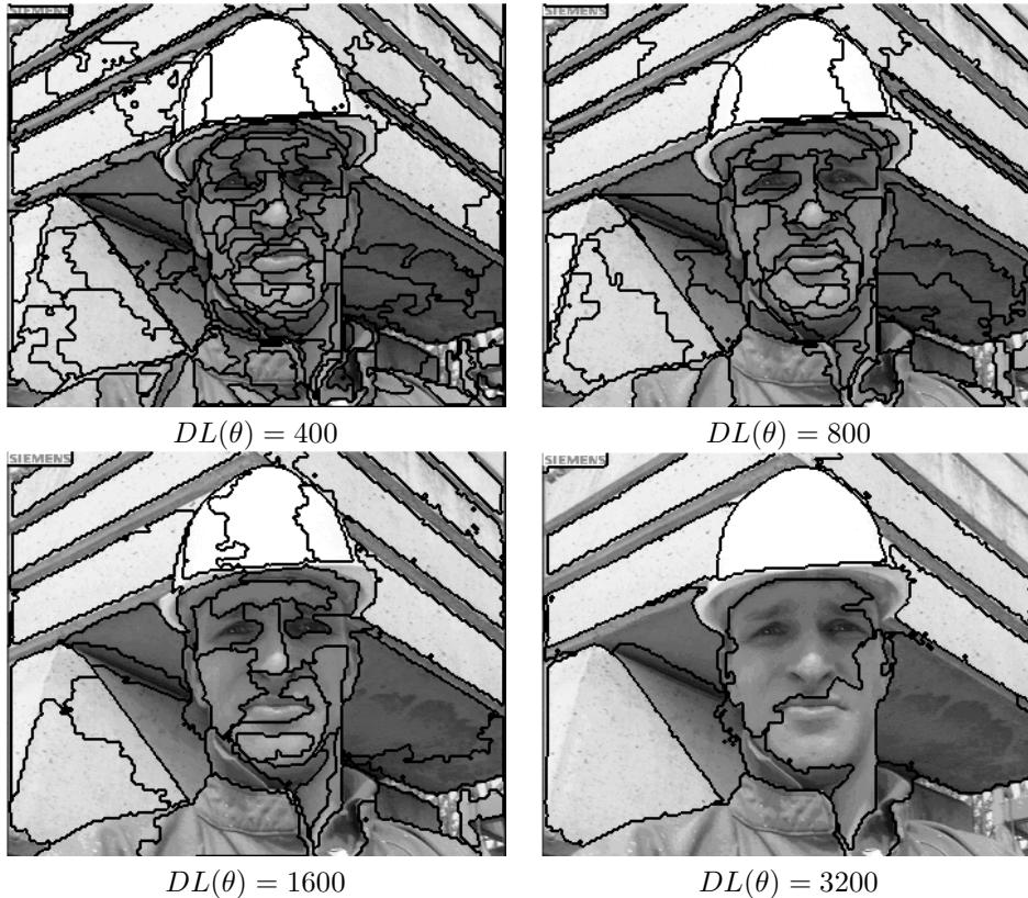
Figure 2. Example of spatial segmentation with different levels of details. Segmentation are obtained with different values of the penalizing cost ( DL(\theta) in 9 ).
