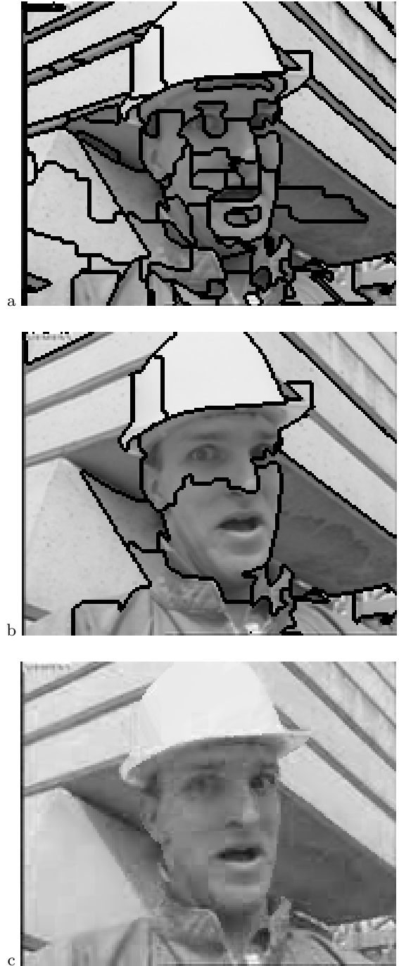
Figure 6: Results obtained of frame 96 of Foreman sequence: initial spatial segmentation (a), final segmentation obtained (b), decoded frame (c).
