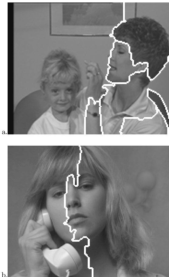
Figure 7: Examples of segmentations obtained that are not suited with the boundaries of the objects present in the scene. (a) Mother&Daughter sequence, the hand and the girl are not segmented and parts of the woman are merged with the background. (b) Suzie sequence, the regions obtained do not correspond to objects of the scene.
