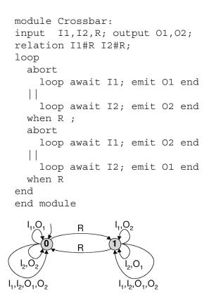
*Figure 3.* A small synchronous program, meant to model a small communication crossbar, and its LSTS. We omitted stuttering reactions and  $\perp$  values.
