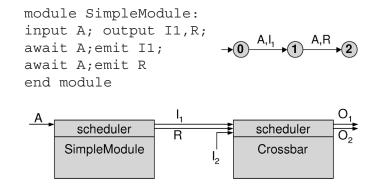
*Figure 4.* The SimpleModule synchronous module, its LSTS (top left), and a small GALS system (bottom) formed by composing SimpleModule and Crossbar
