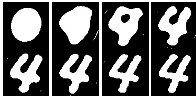
Figure 12: Progressive synthesis of the image of a digit 4, using its Zernike moments of order up to 2, 6, 8, 10, 12, 14, 18 and 20
